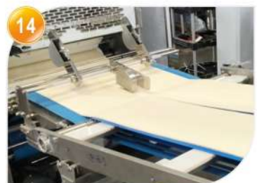
14 第三道厚度成型桿壓 Finally thickness kneading process
