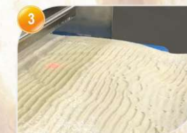
3 自動導麵設計(汽缸切斷傳動) Auto dough guiding design (Cylinder cutting transmission)
