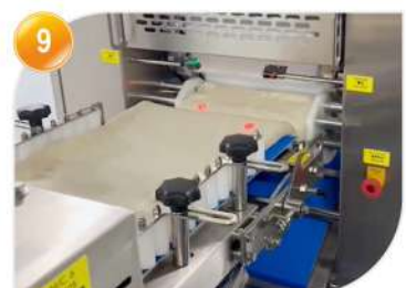
9 入麵輸送→桿壓 Deliver dough sheet, ready for kneading
