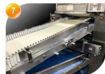
7 麵帶壓麵 (PLC伺服傳動控制) Dough kneading/sheeting process (Servo transmission)
