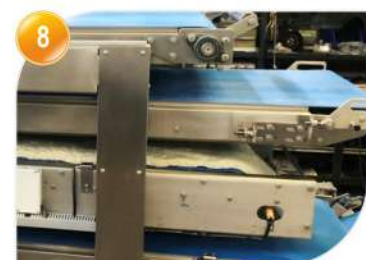
8 滑軌式三層輸送設計 (延長鬆弛時間) Slide rail type three-level conveyor design (Extend resting time)
