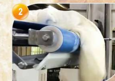
2 麵帶爬升設計 Dough sheet climbing design
