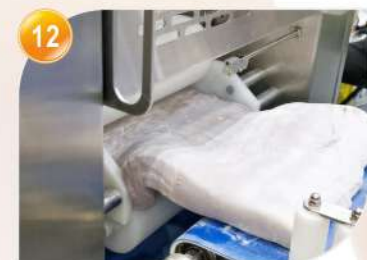
12 第一道輸入麵桿壓 Main first kneading process
