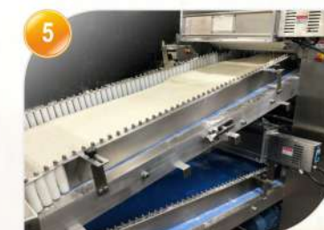
5 麵帶壓麵 (PLC伺服傳動控制) Dough kneading/sheeting process (Servo transmission)
