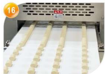
16 伺服切斷傳動 Cutting transmission by servo control system
